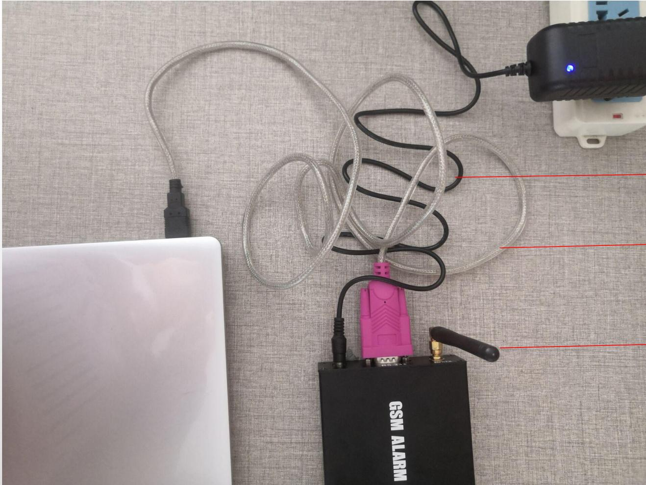
1. Connect the power supply for the gsm receiver.
