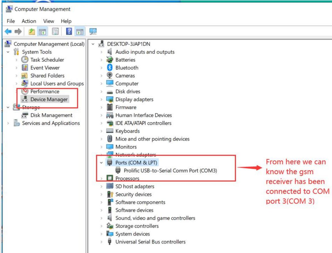
The above operations, you can know the right COM port of the GSM receiver connect to.
