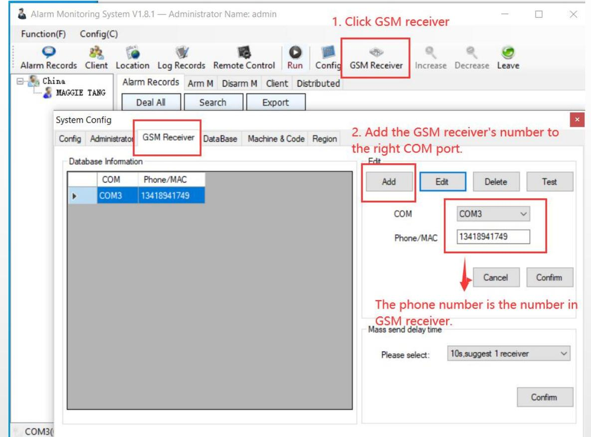
GSM receiver-Add- enter the right COM port - GSM receiver's number. (Refer to step 2.)
