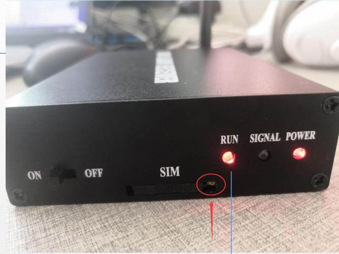
SIGNAL: Blinking every 2s means GSM network is normal
