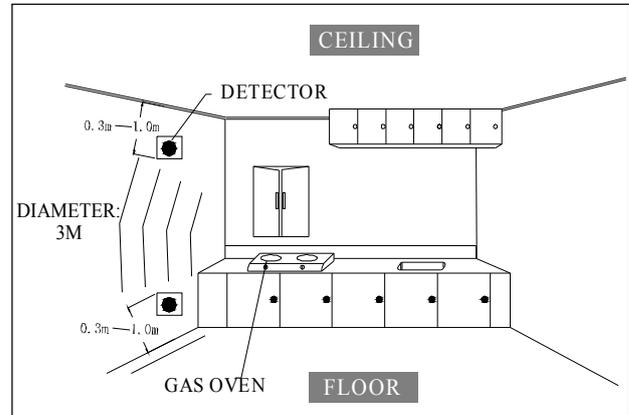
3. Fix the attached installing base into a wall firmly with screws and hang the detector .
